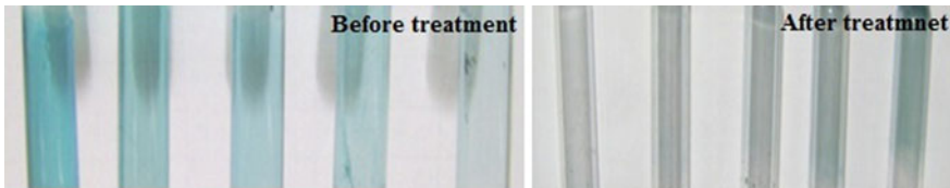
Fig. 4 Thin film of malachite green at various concentrations before and after enzymatic wash. Below tubes shows the residual dye leached out by enzyme solution
