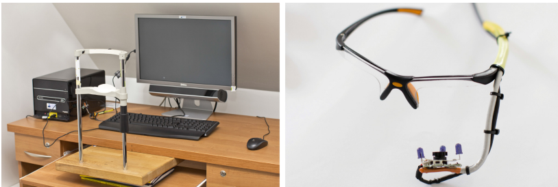
Fig. 2. Left: Hardware setup used for the experiments, RED250 eye tracker is located under the display. Right: DIY eye tracker.
