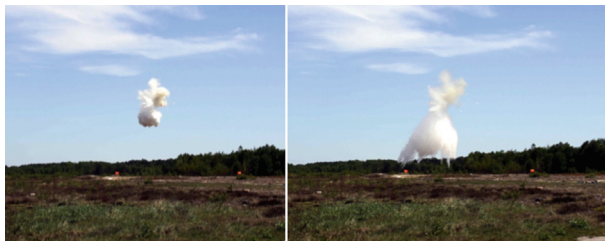
Fig. 8. Explosion of the water-capsule 16 m over the ground - based on the registered film
