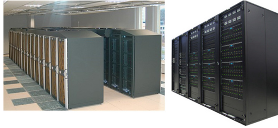
(a) Hardware basis: High Performance Computing Cluster MARS SGI Altix 4700 @ TUD with 1024 cores possesses the performance 13,1TFLOPS
