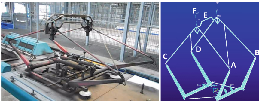
Fig. 1 Pantograph under consideration; left a picture (courtesy of Trenitalia); right FEM model
