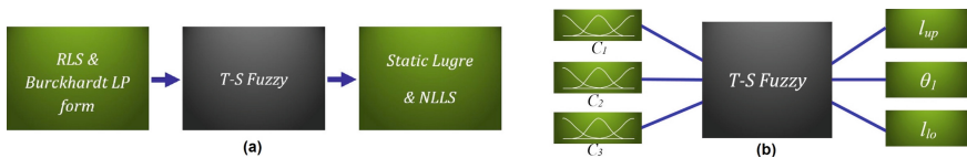
Fig. 2 Proposed algorithm architecture (a), and the Fuzzy logic based parameter conversion (b)
