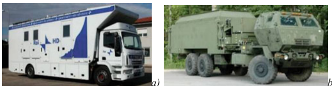
Fig. 3 a Mobile remote broadcast television studio; b Military shelter on truck
