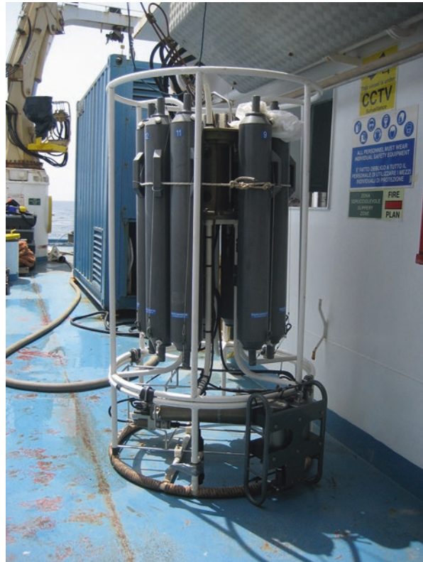
Fig. 2.1 The picture shows the equipment generally used for sampling of brine and interface from DHABs during oceanographic cruises. Niskin bottles of 10 L capacity are located on a rosette sampler equipped with conductivity-temperature-depth (CTD) and pressure sensors
