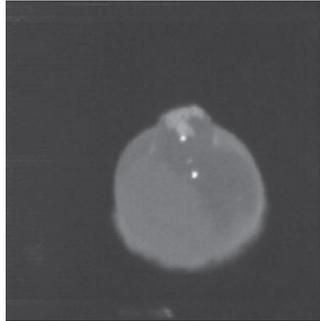
Figure 2. Quench of a Fe<sub>50</sub>Co<sub>50</sub> sample. The video captured the recalescence of the sample as can be seen by the lighter gray region that will eventually engulf the entire sample. The lighter portion at the top of the sample is an oxide.
