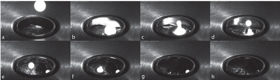
Figure 3. Rapid quench sequence of a Fe<sub>50</sub>Co<sub>50</sub> alloy from (a) start of drop, to (h) end of quench.
