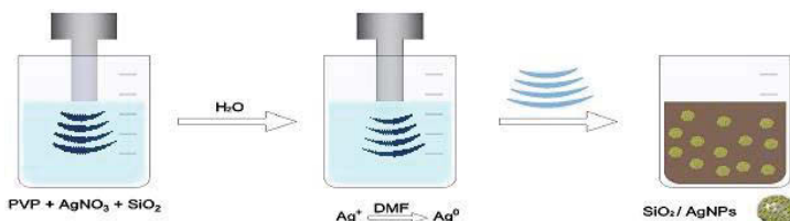
Figure 1. Schematic diagram illustrating the synthesis process of the silver decorated silica ( \text{SiO}_2 / \text{Ag} )
