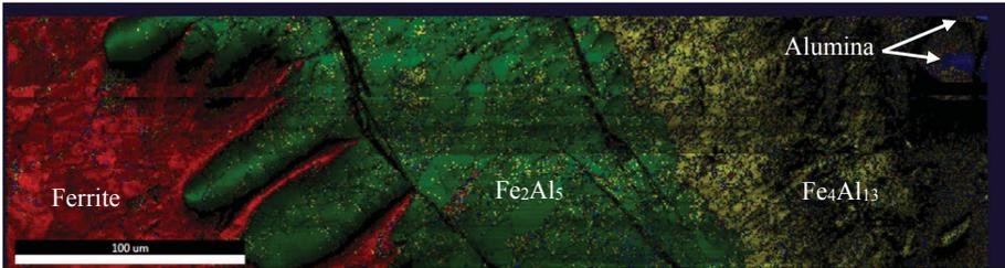
Figure 6. EBSD phase map of the A36/Al-Al<sub>2</sub>O<sub>3</sub> interface.
