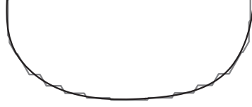
Figure 2: Lower half of a dislocation loop obtained from microMegas (gray) and corresponding spline fit performed by D2C (black).
