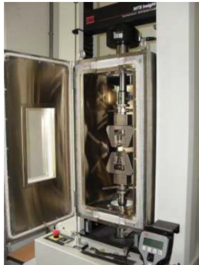
Fig. 1 left) The four SMA samples employed for the mechanical characterization; right) Tensile test machine with environmental chamber.
