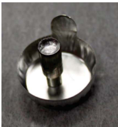
Figure 4. Quench vessel filled with a gallium-indium alloy (61Ga 25In 13Sn 1Zn).
