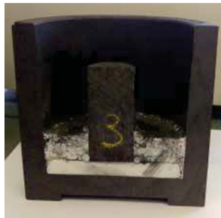
Figure 4. Section of the crucible after two hours of electrolysis for the experiment with the bath sample containing 0.16% carbon
