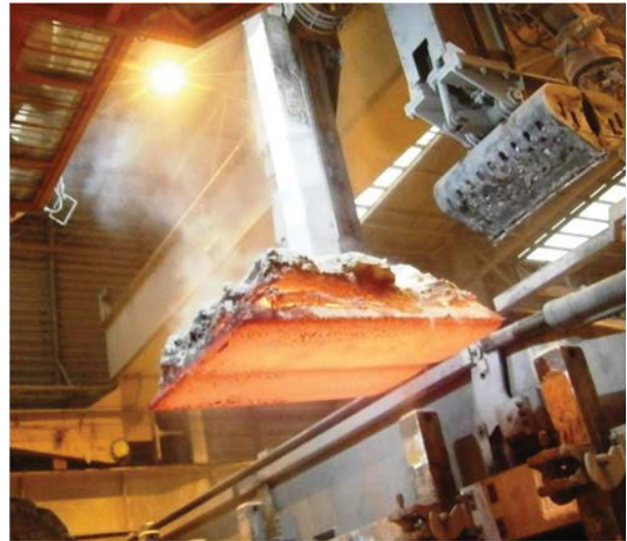
Figure 2: Long anode that is evenly consumed
