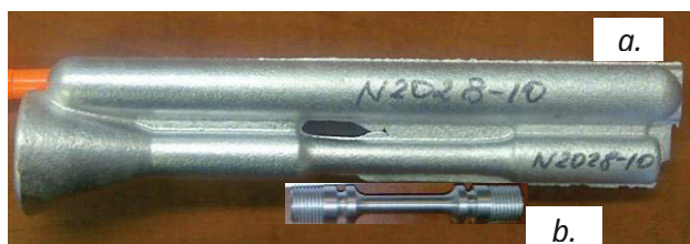
Figure 1. The aluminum test bar (a.) cast using ASTM B108 steel mold and machined creep specimen (b.). Total length of the specimen is 80 mm, with the length of the gauge section of 32 mm.
