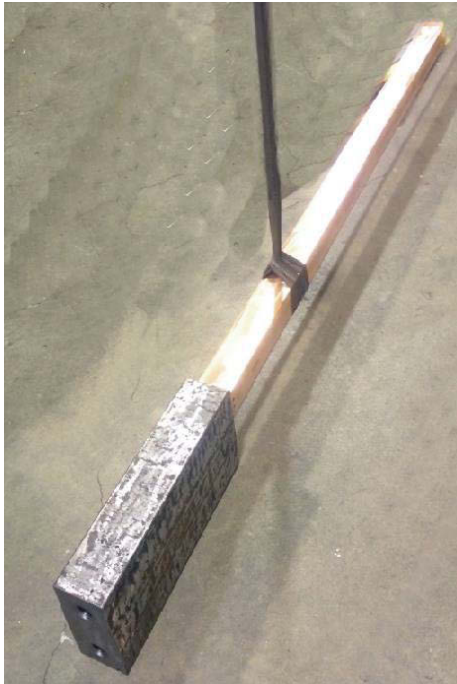
Figure 12: Copper bar coupled to a steel bar
