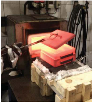
Figure 2: Box at 900°C containing the sample
