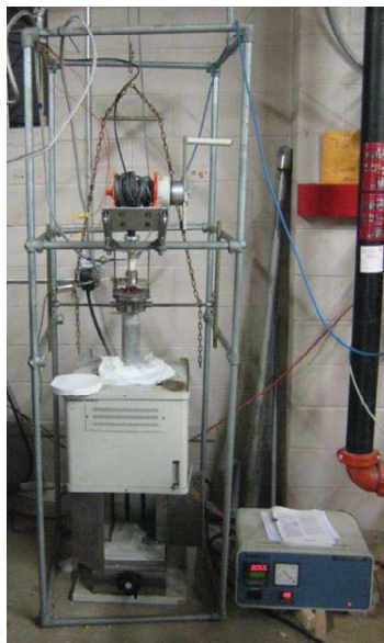
Figure 1: LIBS Probe Immersed in the furnace [16].
