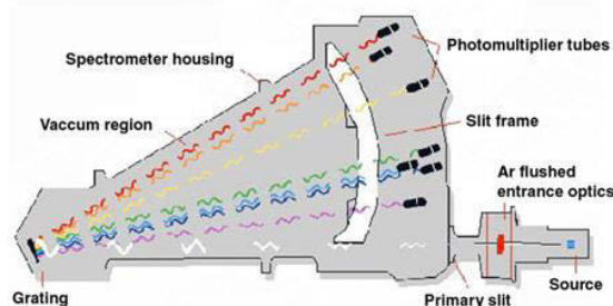
Figure 3: Wavelength emitted is specific for each elements present in the sample
