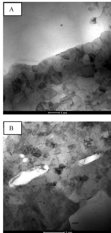
Fig. 3 TEM microstructure of the interlayer: a) on the side of the AZ91 magnesium alloy, and b) on the side of the 6101 aluminium alloy.
