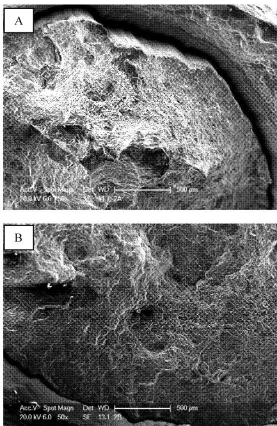
Fig. 7 Rods fracture topography after the extrusion of feedstock with plating thickness of a) 5 mm and b) 3mm.
