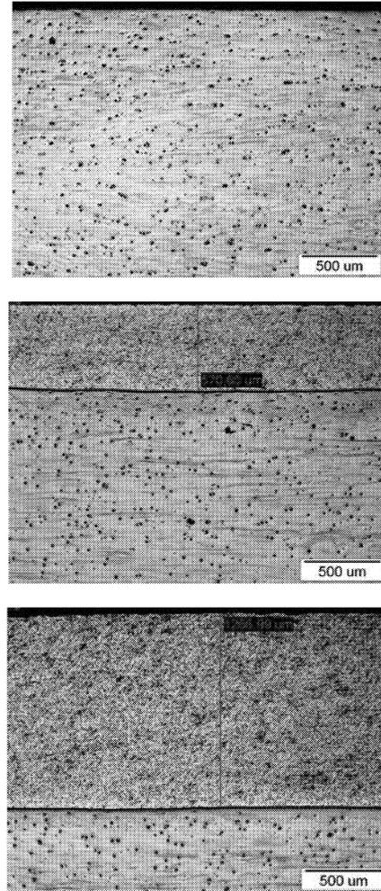
Fig. 6 Microstructure on the rod cross-section with the coating of 3 mm thickness: a) the starting part, b) the middle part, c) the end.
