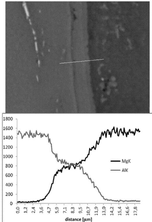
Fig. 1 Chemical linear analysis of the interlayer in samples after compression.
