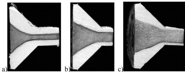
Fig. 5 Cross-sections of the end parts of the successive sample extrudates with the coating thickness of: a) 5 mm, b) 3mm c) 1 mm.
