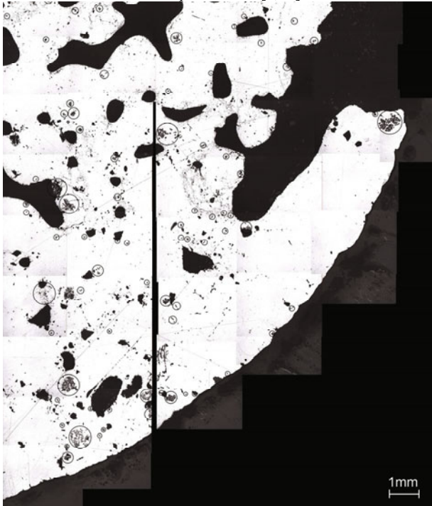
Figure 11. Transversal metallographic cut of a quarter of the filter (100µm from the filter inlet)
