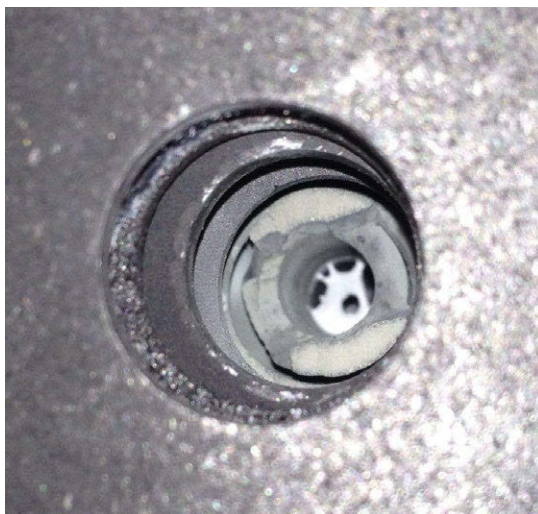
Figure 3. Condensation of SiO 2 inside optical access tube.
