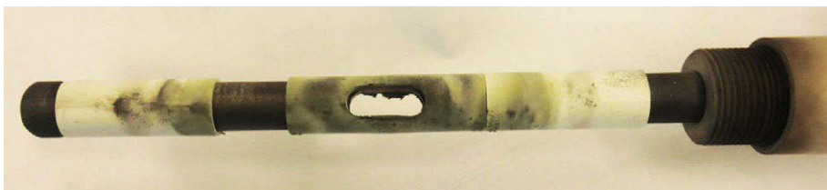
Figure 4. SiC condensation on the BN sleeve of the optical access tube.
