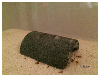
Figure 1. An image of the susceptor used for microwave annealing.
