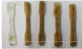
Figure 3. Typical tensile ruptured specimens volume fraction of malva reinforced polyester composites.
