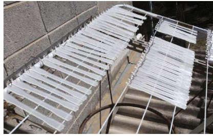
Figure 1. Device with dumbbell samples for environmental ageing exposed outside at the polymer processing laboratory IPEN/CQMA.
