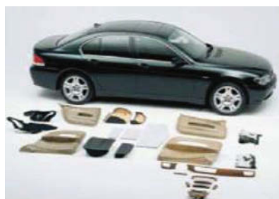
Figure 1. BMW sedan and its different parts made of polymer composites reinforced with lignocellulosic fibers. ( www.bmwgroup.com )
