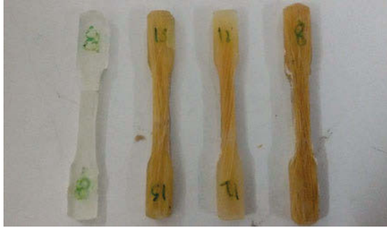
Figure 4. Samples with 0, 10, 20 and 30 % in volume of Figue fiber.
