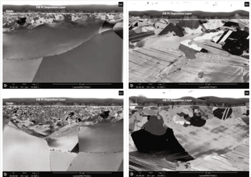
Figure 3. FIB cross sectional images of SCW tested specimens. (a,c) “as-received” sample; (b,d) rolled sample
