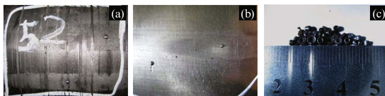
Fig. 1 Photos of buildups embedded in the surface of carbon sleeve in low temperature zone (a) and high temperature zone (b) of annealing furnace; (c) buildups in different shapes and sizes.
