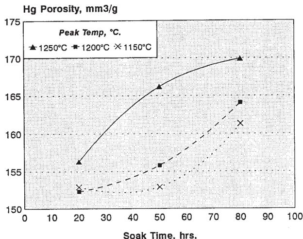
Figure 4. Anode porosity, as determined by porosimetry, as a function of peak temperature and soak time.
