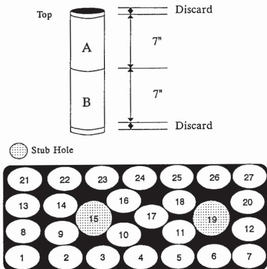
Figure 1: Core sampling pattern within the anode
