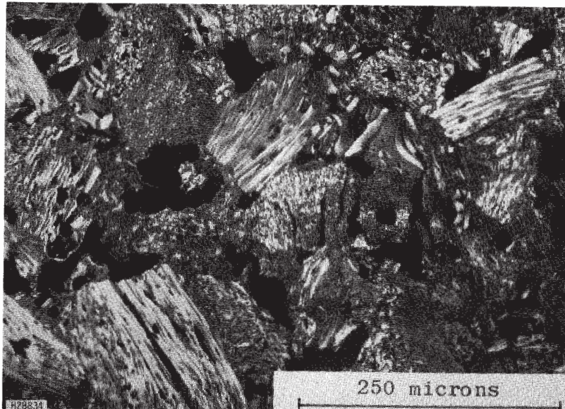
Figure 9 Microstructure of Baked, Well-Mixed, Compacted Anode Paste
