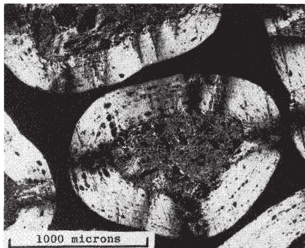
Figure 13 Microstructure of Pyrocarbon-Coated Fluid Coke
