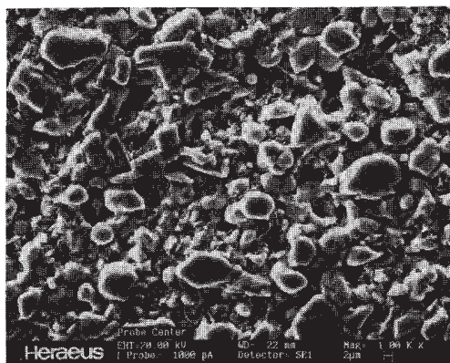
Figure 6: Secondary electron scattering image of sample 5 after heat-treatment. The picture is taken in the centre of the coating.
