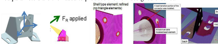
Figure 4 Failed bracket load distribution, mesh configuration and assumptions
