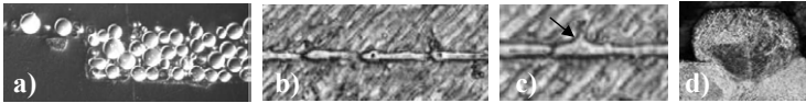
Fig. 4: a) powder bed at a 90µm high stair, b) Rayleigh effect, c) melt pool pinned on particle, d) melt pool cross-section (shape caused by surface tension)
