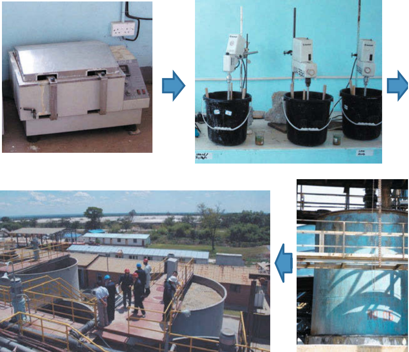
Fig. 6 6-stage enlarge cultivation of bioleaching bacteria in Chambishi.
