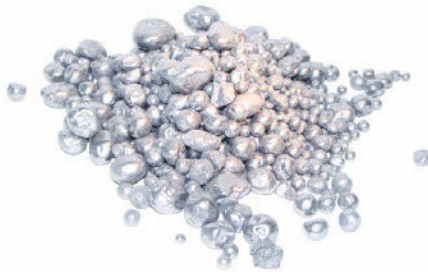
Figure 8 – Typical beryllium pebbles produced in the Materion Pebbles Plant.
