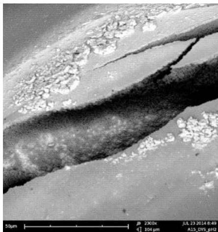
Figure 5: Polystyrene Resin Rupture Showing Interior Loading
