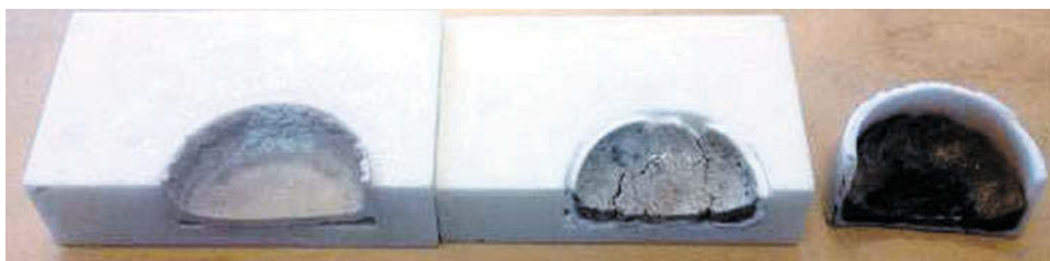
Figure 6. Crucibles after saturation experiments. From left to right are YSZ, SiO 2 and Al 2 O 3 crucibles. ZrO 2 and SiO 2 crucibles are embedded in part of the holding block, which was made of alumina.
