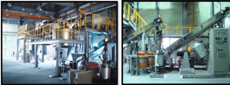
Figure.9. 200 kg/hour MSWI bottom ash multi-process Figure.10. 20 tonns/hour Removal process model of heavy metals chlorides from MSWI bottom ash
