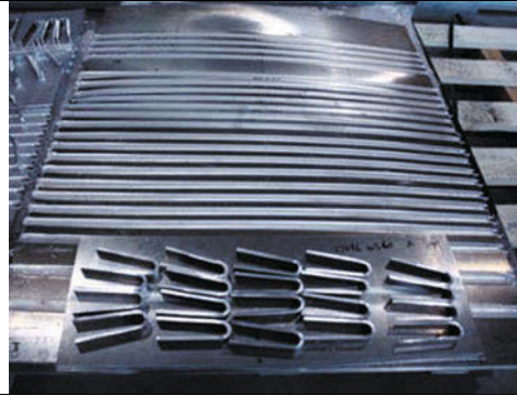
Figure 10 Tool life trials when welding 6mm thickness AA5083-H111
