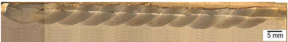
Figure 3: Macrograph showing the cross sectional view of overlapping FSP passes
