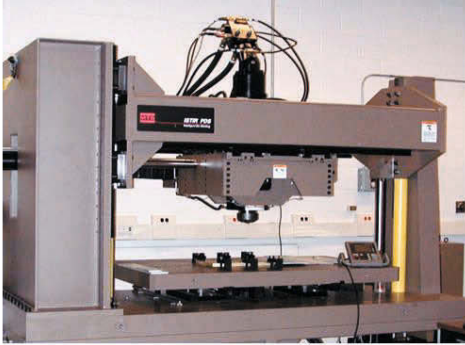
Figure 11: Proposed DLA-FSW system consisting of (a) traditional FSW setup and (b) combined FSW setup with the HPDL setup used in this research. The HPDL used in this setup (including the mounting components used) have been designed to mount to the traversing head of the already existing FSW setup shown in (a).
