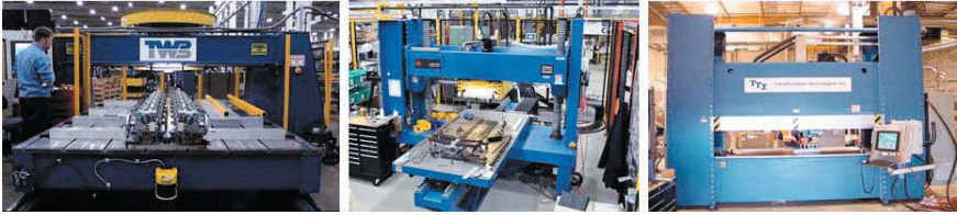
Figure 1. Visual Comparison of FSW equipment utilized for this study. High Speed FSW System at TWB LLC (left), R&D Machine at GM Technical Center (center), and R&D Machine at PNNL (right).
