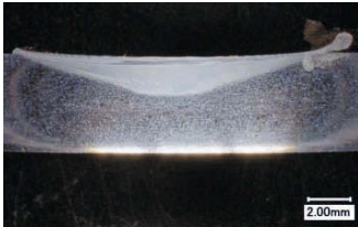
Figure 6. Cross-section of a FSW on AISI304 (2mm probe length).
