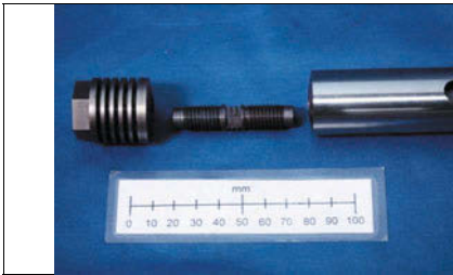
Figure 2a Tool components: bottom shoulder, probe and top shoulder
