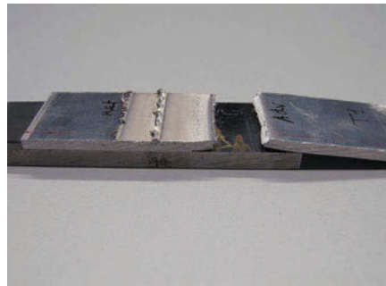
Figure 8: HAZ failure in AA6082-T6 HAZ (sample “FSW 3passes”).
