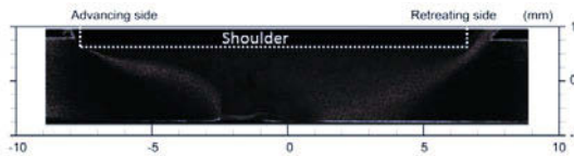
Figure 8 Macrostructure of friction stir weld.
