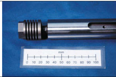
Figure 2b Bobbin tool as assembled
