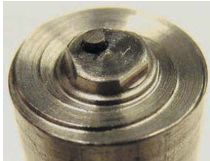
Figure 2: Friction Stir Scribe (FSS) Pin tool
