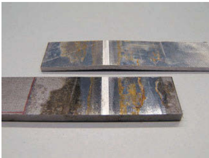
Figure 7: Interfacial failure in the Al-Fe interface (samples “FSW 1pass” and “FSW 2passes”).
