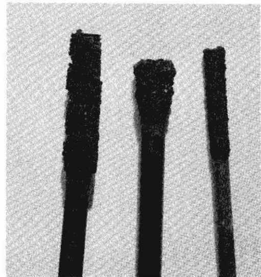
Fig. 6. Carbon deposits on rods made of; 1: iron (3 mm), 2: vitreous carbon (3 mm) 3: tungsten (2 mm). CR=1.50, t=1000°C, total current 1-5 A.
