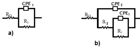
Figure 6. Equivalent circuits obtained from the adjustment of the experimental data. a) Al-1wt.%Cu. b) Al-4.5wt.% Cu.
