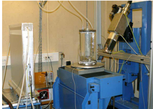
Figure 1: \mu CT setup for analysis of ASR-induced damage processes in concrete
