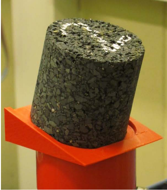
Figure 6: Asphalt drill core during CT measurement
