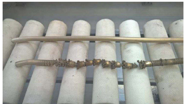
Figure 8: Outcomes of extrusion trials using different container temperatures. A 15°C increase in container temperature lead to hot shorting. A 15°C decrease in temperature resulted in no extrusion.
