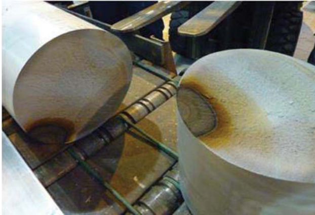
Figure 3: Catastrophic failure of a DC cast billet caused by residual stresses during casting.
