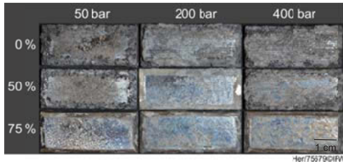
Figure 8. Photos of deep-rolled samples after immersion test. From left to right: increase of process pressure; from top to bottom: increase of overlap.
