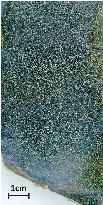
Fig. 5. AZ31 Mg-alloy ingot cast after application of intensive shearing, showing fine and uniform grain structure upon final solidification.
