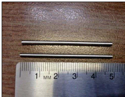
Figure 1. Specimens for three-point bending corrosion fatigue tests
