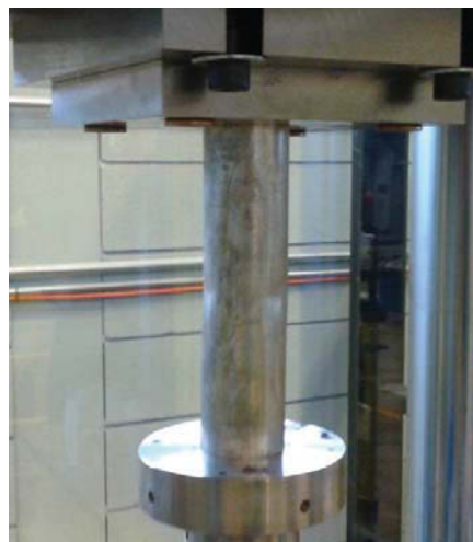
Figure 4 – Experimental setup for an axial crush test being performed on a thin-walled tube component.
