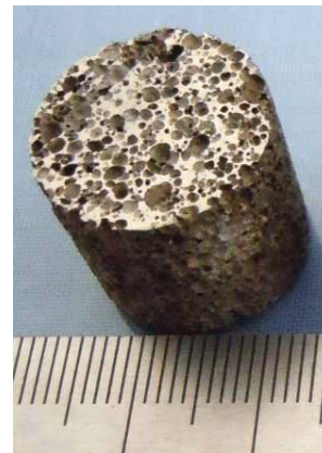
Figure 1. A cylindrical Mg foam specimen fabricated by the direct foaming process.
