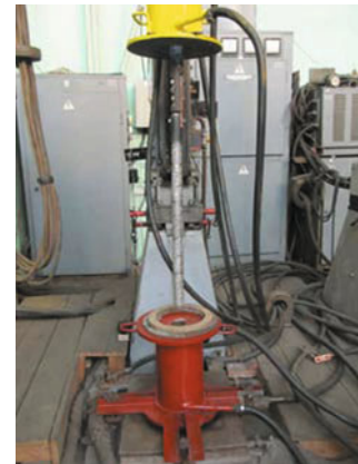
Figure 4: The chamber electroslag furnace A-550 (724 kW) The remelting was conducted under a flux of pure CaF 2 (TU 6-09-5335-88). The flux was melted directly in the crucible, using the technology of "solid" start. The starting mixture was prepared of titanium chips and the operating flux. The electrical parameters of the refining maintained at U = 36.0 V and I = 2.0-2.5 kA, providing a good surface quality of the remelted ingots (Figure 5).
