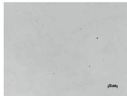
Figure 6. Nonmetallic inclusions distribution in ESR hollow ingot, 50\times .
