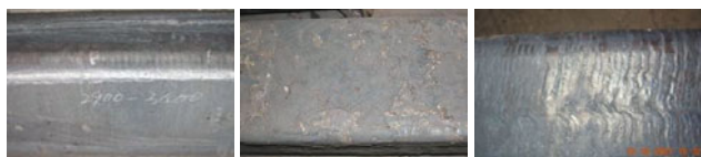
Figure 1. Surface quality of 300×340×6000mm ingot.
