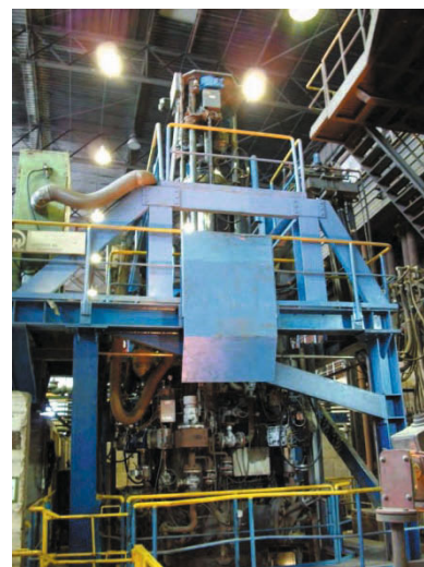
Figure 1. View of the PESR furnace at Energietechnik Essen GmbH for ingot weight up to 20 t and diam.1030 mm.
