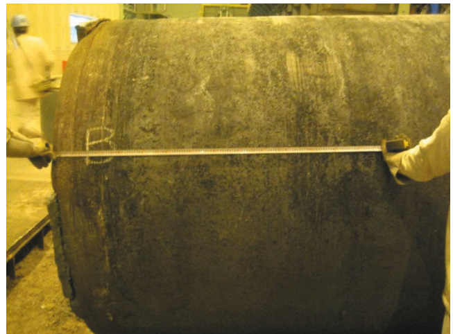
Figure 3: Bottom Part of a 1.900mm dia. ESR ingot produced in a 145t short collar mold ESR plant at Japan Casting & Forging Corporation. The bottom part shows a rectangular appearance without any unmelted slag and the surface is smooth.
