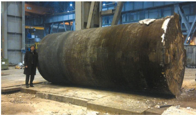
Figure 6: Heavy forging ESR ingot with a weight of 250 tons and a diameter of 2600mm produced in a 250ton static mold ESR plant at Forgiatura A. Vienna. The surface is smooth over the whole ingot length, due to a very stable remelting process with well controlled electrode sequences.
