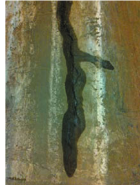
Figure 4. The surface crack of ingot
