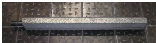
Figure 6. Pressed Ti-45Al electrode made from titanium sponge and aluminum rods
