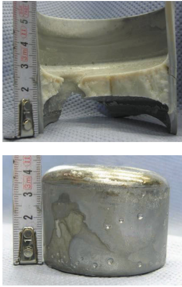
Figure 8: Representative illustration of the received slag layer attached to the crucible (up) and the obtained metal ingot (down)
