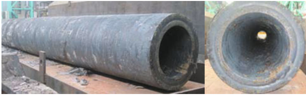
Figure 3. Appearance of hollow ingot of \Phi 650/450\text{mm}\times 6000\text{mm} .
