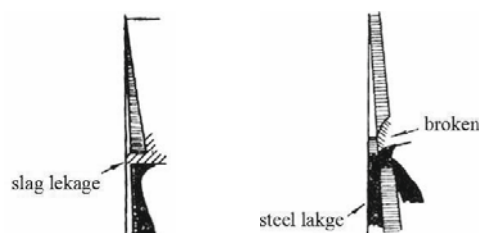
Figure 3. The fundamental of slag broken due to the friction.
