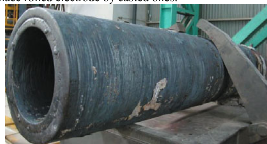
Figure 6. ESC TC hollow ingot produced with electrode change
