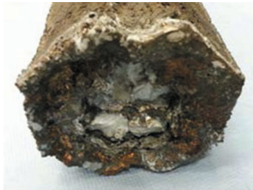
Figure 9. Electrode tip after remelting with calcium addition
