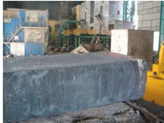
Figure 3. Surface quality of remelted slab ingot.
