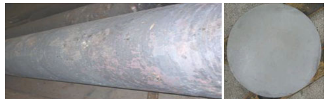
Figure 7. Surface quality and inner macroscopically quality of Φ600×6000mm ingot.
