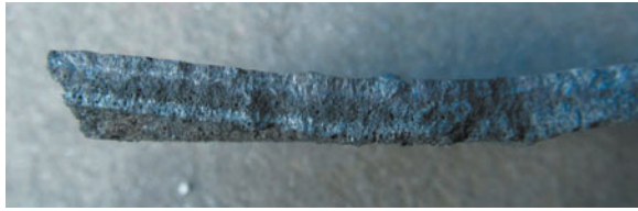
Figure 6: Frozen Slag Layer From in Front of Semigraphite Bricks
