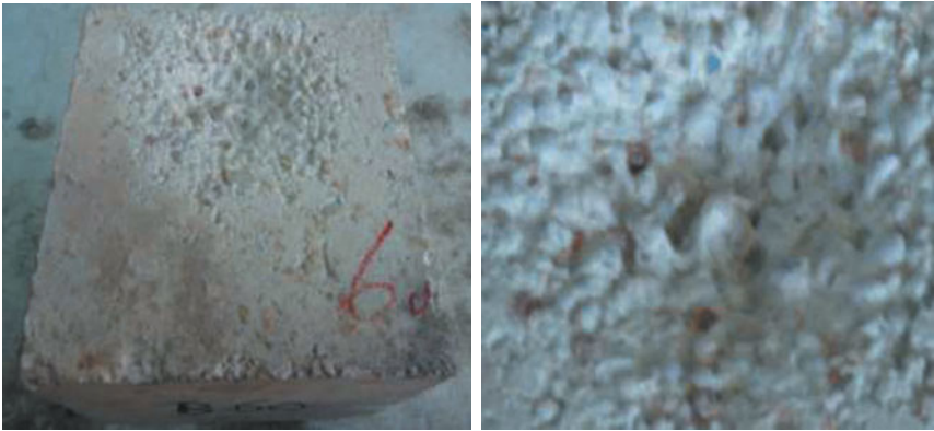
Figure 4. Surface morphology of mullite brick at cooling section after wear
