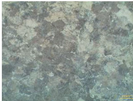
Figure 6. Schematic diagram of pearlite and sorbite in wire rods
