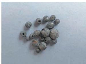
Fig. 2 Photograph of metal balls recovered at the cathode
