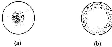
Fig. 11.7 Effect of directional emissivity on the appearance of radiating spheres: (a) electrical conductor with brighter periphery; (b) electrical insulator with dimmer periphery.
