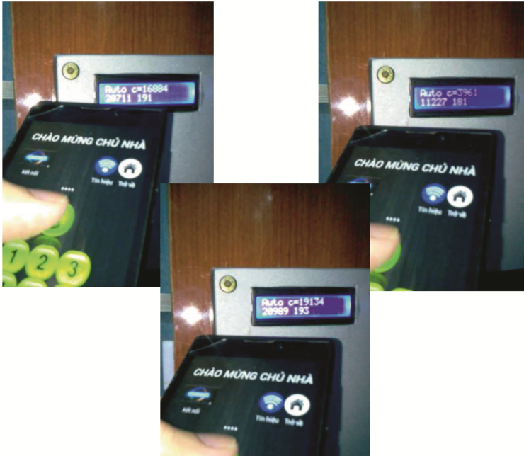
Fig. 8. Three continuously pressing open button with the same password (from left to right: ciphertext is 16884, 3961, 19134)
