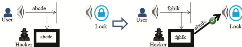
Fig. 1. Jam and relay attack
