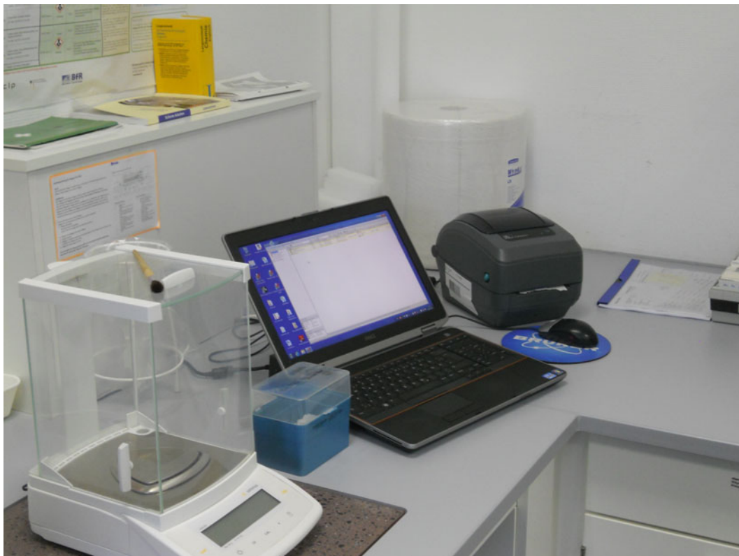
Fig. 4 Labelling of samples from the entering in the analytic laboratory. LIMS, Laboratory Information Management System
