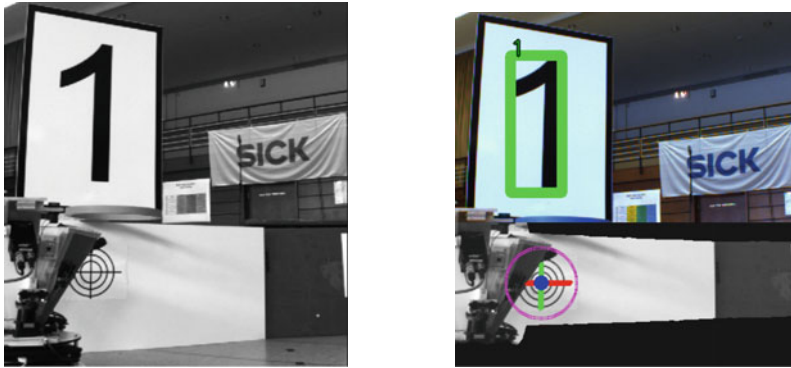
(a) The robot's camera image, showing an occluded bull's eye target and the number sign of station 1. (b) Overlay of the detections of two dataflow graphs, one detecting numbers and one detecting bull's eye targets.
