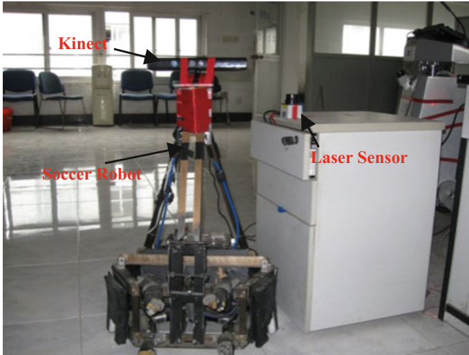
Fig. 7 Robot and the sensors used in the experiment
