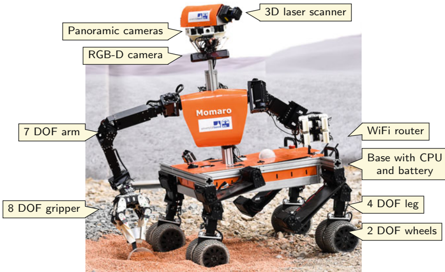
Fig. 1 The mobile manipulation robot Momaro taking a soil sample
