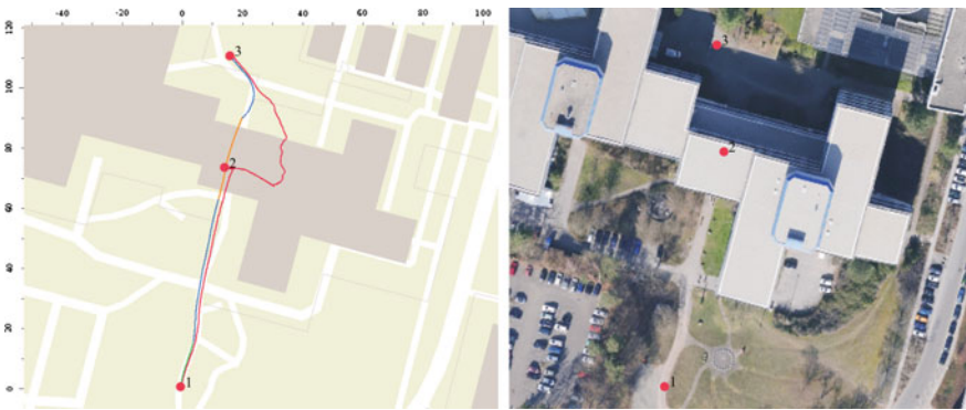
Fig. 5 The vehicle drove from point 1 to point 3 with an intermediate stop at point 2. As the stop is lying inside a tunnel, the GPS-measurements (red line) are heavily drifting. The output of the filter is segmented in multiple stages: no influence part (green), influence part with an increased variance in the localization filter (blue) and a yellow part, where the GPS measurements are not incorporated at all
