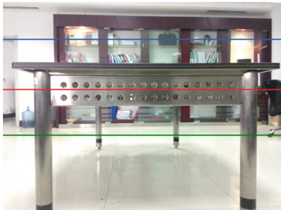
Fig. 1 Obstacles in complicated 3D environment: if we cut the 2D slice like the red line , the table will be considered as an obstacle when creating the 2D GVD. However, if we cut the 2D slice like the green line or blue line , it will be considered as free
