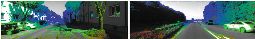
Fig. 3 Computed semi-dense depth maps for KITTI datasets (sequences 00 and 01). Color depicts estimated distance to the sensor
