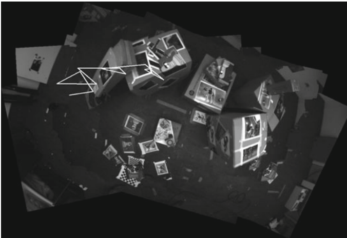
Fig. 3 Image Stitching process during a rototranslation of the robot. Dataset taken from http://rpg.ifi.uzh.ch/software_datasets.html
