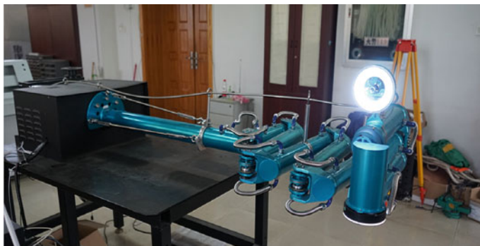
Fig. 1 The snake-like robot for inspecting tokamak vessel
