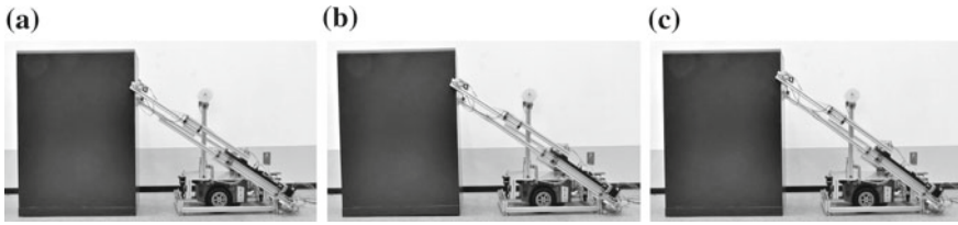
Fig. 9 Slippage between the end-effector and an object being pushed by the robot
