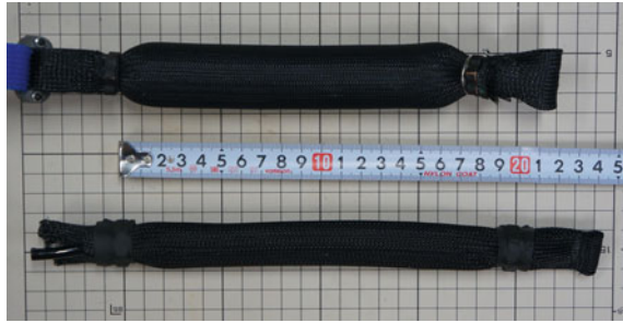
Fig. 2 Artificial muscles in the robot. With supply ( upper ) shows the length of 18 cm, and without supply ( below ) shows the length of 20 cm
