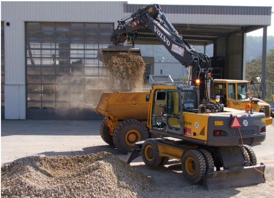
Fig. 1 The bucket excavator Thor during autonomous truck loading
