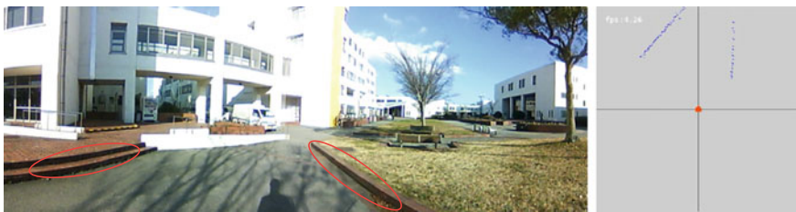
Fig. 9 Detection of low steps. A local obstacle map centered at the current robot position is shown on the right . Red ellipses on the left show the detected step locations
