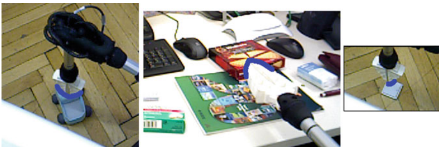
Fig. 5 Some cases in which colour-edge combination is not enough for properly evaluating the grasping task such that the blue line corresponds to the detected contact points
