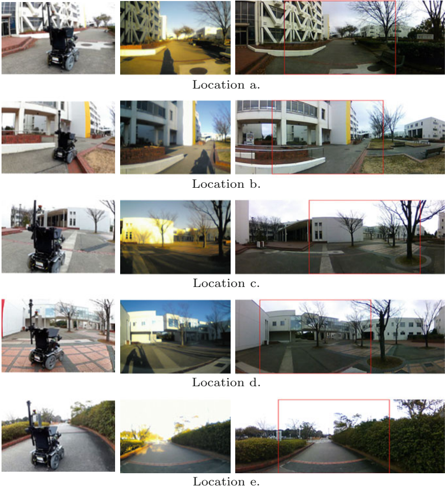
Fig. 11 Navigation experiment. Left Robot in motion. Center Estimated location (i.e., best matched training image). Right Input image and selected moving direction
