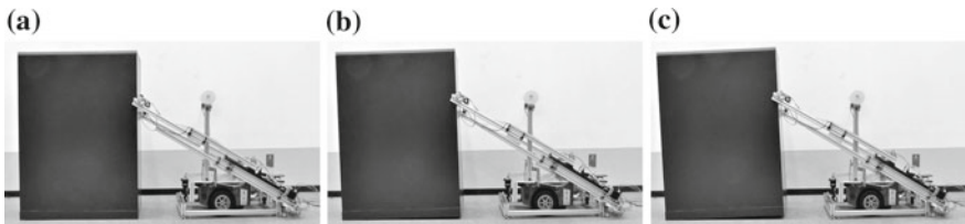
Fig. 11 Slippage between the outrigger and ground while the robot pushed the object
