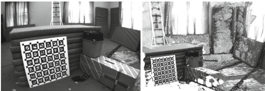
Fig. 6 Left Camera image. Right Reconstructed semi-dense 3D point cloud
