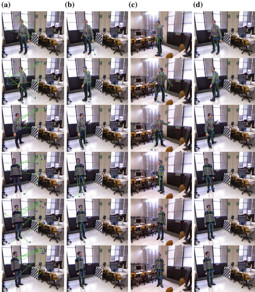
Fig. 5 Some sample frames of the dataset we used for testing the proposed approach. Each row represents a frame. The different columns represent: a [2] on the C_0 stream; b ours with PD and JT on the C_0 stream; c ours with PD and JT on the C_1 stream; d our multi-view approach re-projected on the C_0 camera
