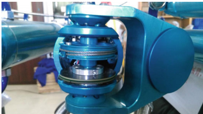
Fig. 7 Joint equipped with absolute position sensor
