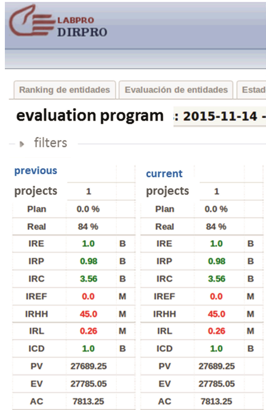
Fig. 3. Indicators, some of them included in the PMBOOK standard, which are used for automatic assessment
