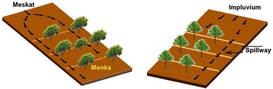
Fig. 10 The Meskat and Menka type water harvesting system in Tunisia (Source: http://www.rainwaterharvesting.org )
