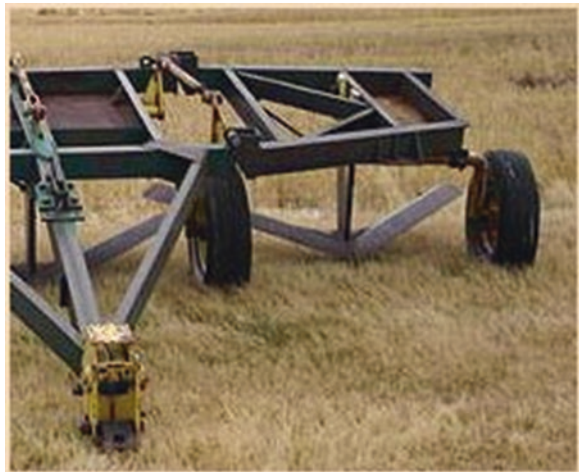
Fig. 2 Noble blade plow that ran about 10 cm below the soil surface to till the soil to cut roots of weeds without depriving the land of surface trash and standing stubble
