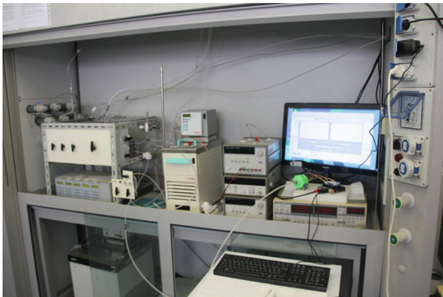
Fig. 4 The gas control setup
