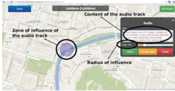
Fig. 11.5 The monitoring tool allows creating context based audio tracks. Every time the user enters the operational range of each audio track the tool notifies the user with the corresponding audio track. University of Deusto
