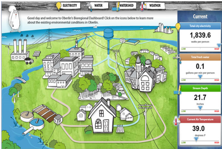
Fig. 7 Citywide dashboard. An animated display of real-time electricity and water use and environmental conditions in entire communities or organizations. Gauges and animations of water flowing through pipes and electrons flowing down power lines reveal how decisions made in our homes and workplaces are reflected in city-wide patterns and conditions. Messages delivered by “Wally Walleye” and “Flash the Energy Squirrel” narrate the story of current resource use. Real-time data for the displays are accessed directly from the public electrical and water utility companies. The goal is to situate individual decision-making in a community and systems context
