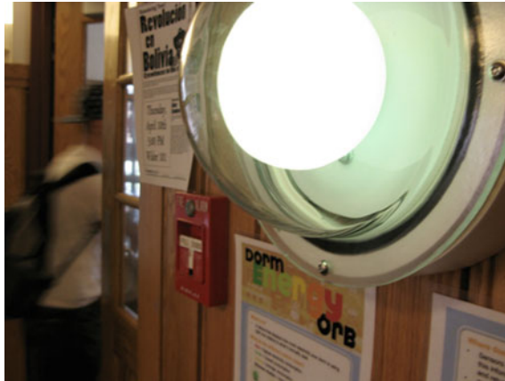
Fig. 4 “Environmental Orbs” glow different colors and with different pulsing patterns to communicate whether current levels of electricity and water consumption within buildings are high or low relative to typical levels of use at this time of day. The one pictured is installed in the lobby of a student dormitory
