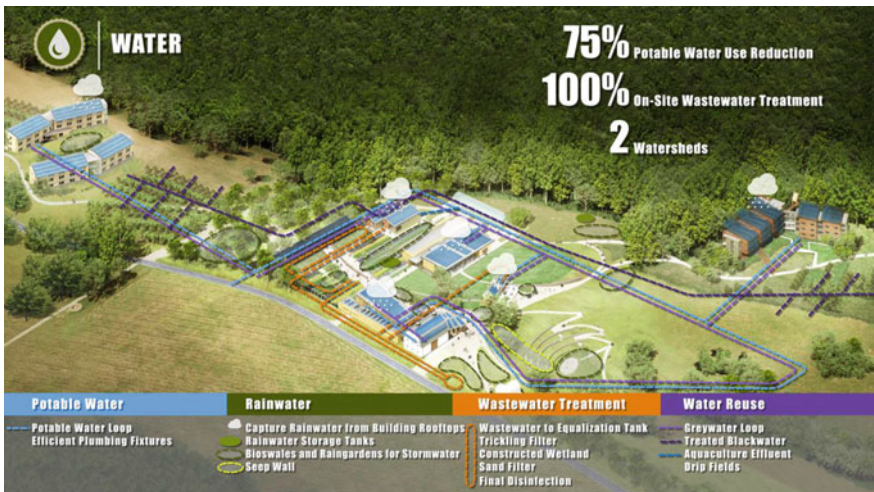
Fig. 4 Diagram of campus water systems illustrating rainwater infiltration areas, rainwater collection and reuse, and onsite biological treatment of waste water for non-potable reuse
