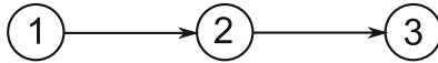
Fig. 1. A directed graph consisting of three nodes. An edge’s direction determines the influencer-influencee relationship. In this case, node 2 is influenced by node 1, but not node 3.
