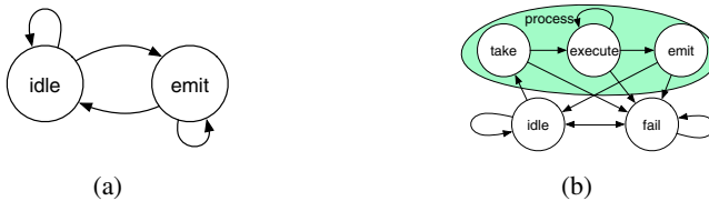
Fig. 3. Finite state automata describing the states of spout (a) and bolt (b).
