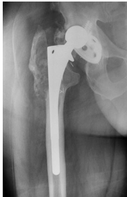
Fig. 7 An AP radiograph of a hip replacement where the head has worn through the metal socket of the acetabular implant. This was more common with older polyethylene liners with poor wear characteristic. This leads to metallosis, an extensive infiltration of pericapsular tissues with black metal debris
