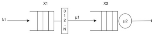
Fig. 17.5: Graphical representation of the tandem queue with batch service in the first queue
