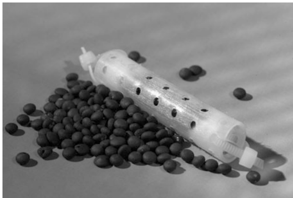
Fig. 13.5 BACTRAP with activated carbon bead figure (Courtesy from André Künzelmann/UFZ)
