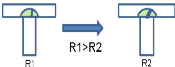
Fig. 31 Formation of a conduction filament in amorphous GST during set pulse. Lower resistance values correspond to larger filament size
