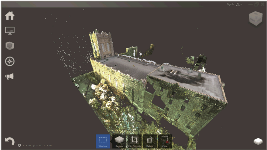
Fig. 8. Combination of the different point clouds acquired through photogrammetry and 3D laser scanning. Software employed: Autodesk Recap.
