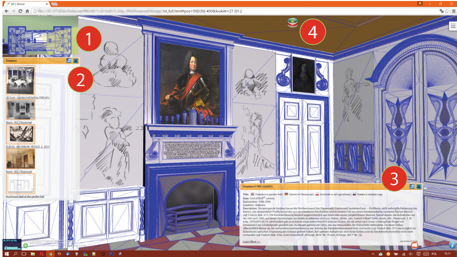
Fig. 12. Prototype of the Virtual Museum: Integration of interactive semantic 3D objects in WebGL. (1) The real-time rendered map of the surroundings with user's focus area and position; (2) Visual information; (3) Metadata and textual content; (4) Paronomic view option.
