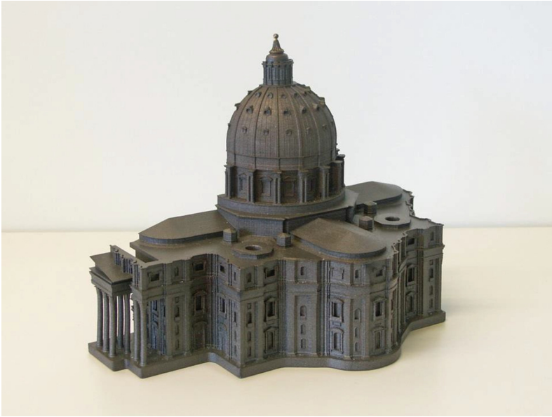
Fig. 30. Saint Peter's Basilica in Rome, metal-printed model (© Technische Universität Darmstadt, Digital Design Unit)
