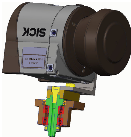
Fig. 9. Rotatable mounting of LMS111 on axis with pair of ball bearings inside sleeve
