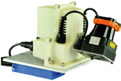
Fig. 7. LRF mounted on the horizontally oriented axis [2]
