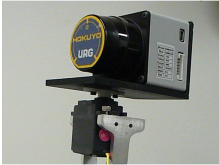
Fig. 5. First know design of 3D LRF with servo [8]
