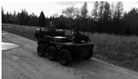
Fig. 5. Unmanned Ground Vehicle TAROS v2. The scanned data is used as a starting basis for the calculation of throughput analysis in complex terrain.
