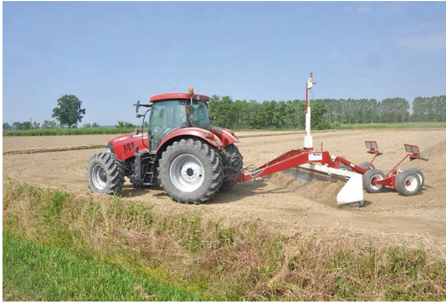
Fig. 4.3 Laser levelling done before sowing of rice
