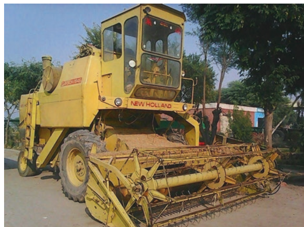
Fig. 16.2 A typical combine harvester for harvesting and threshing of rice crop
